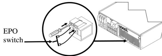
The EPO switch is internally powered by the UPS for use with non-powered switch circuit breakers.
